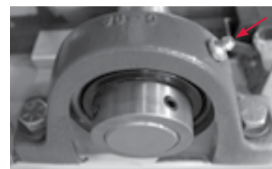
FIGURE 21. Pump grease into two rotor bearing grease points, one on each side of the rotor.
