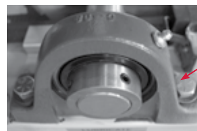
FIGURE 22. Inspect bearing collar to ensure all bolts and screws are tight.
