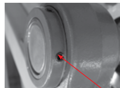
FIGURE 23. The bearing set screws, one on each side of the rotor, should be checked for tightness every six months.
