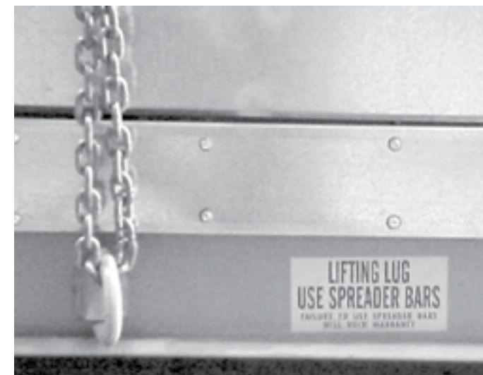
FIGURE 1. Lift modules only with lugs located at the base of each module. Do not use a forklift.
