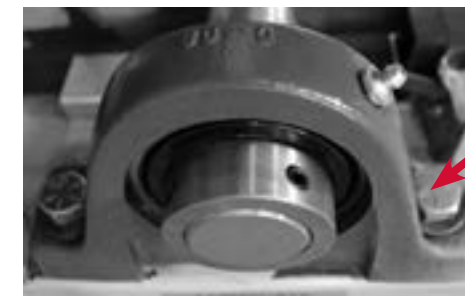
FIGURE 13. Inspect bearing collar to ensure all bolts and screws are tight.
