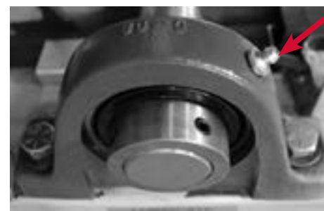
FIGURE 9. Pump grease into two rotor bearing grease points, one on each side of the rotor.
