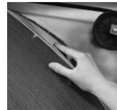
FIGURE 12. Rotate the rotor at least three turns in the direction indicated by the rotation arrow.
