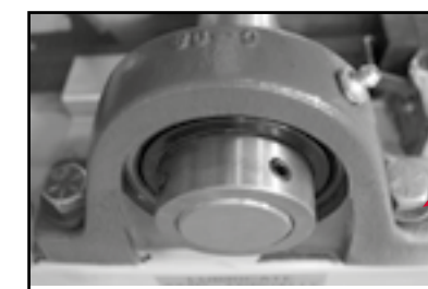
FIGURE 19. Inspect bearing collar to ensure all bolts and screws are tight.
