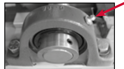
FIGURE 15. Pump grease into two rotor bearing grease points, one on each side of the rotor.
