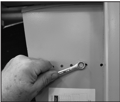
FIGURE 39. To adjust the purge, remove the adjusting bolt.
