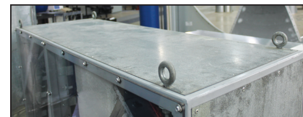
FIGURE 21. Large eyelet lugs atop vertical units should remain attached permanently. However, if they must be removed, be sure to replace the lug with a bolt.
