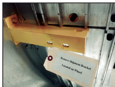
FIGURE 23. Shipping restraint for ribbed rim wheel.
