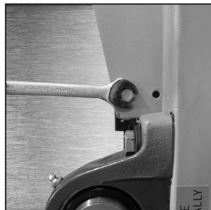
FIGURE 40. After removing the adjusting bolt(s), loosen the bottom pivot bolt.
