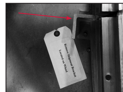
FIGURE 10. Shipping restraint for ribbed rim wheel.
