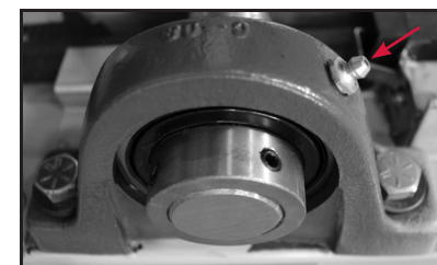
FIGURE 12. Pump grease into two rotor bearing grease points, one on each side of the rotor.
