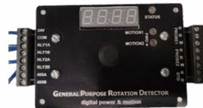
GPRD controller as installed on the electric panel.
