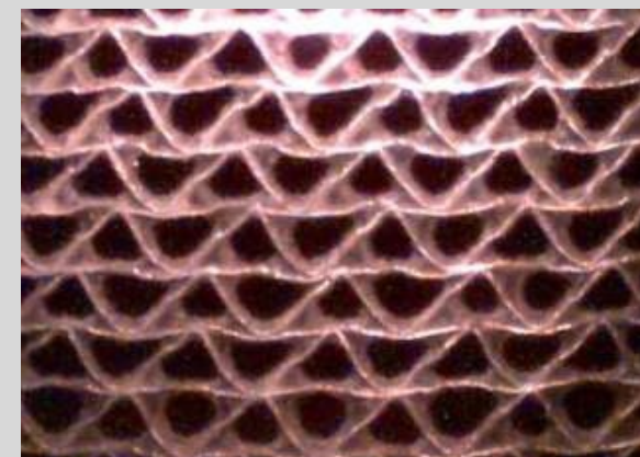
Competitor's small flutes with plugging
