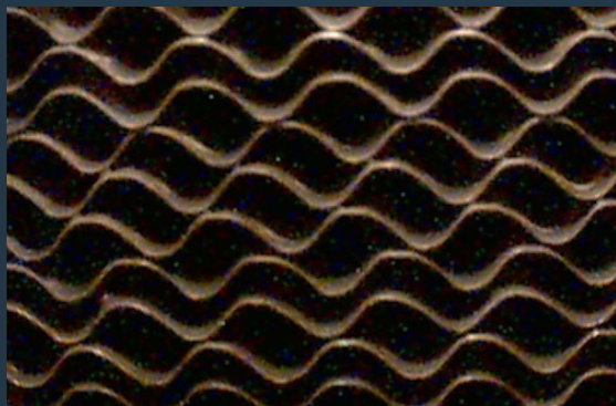
Tobacco build-up on a wheel surface with anti-stick coating face additive.
