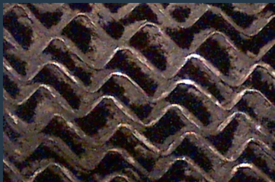
Tobacco build-up on a wheel surface without anti-stick coating face additive.
