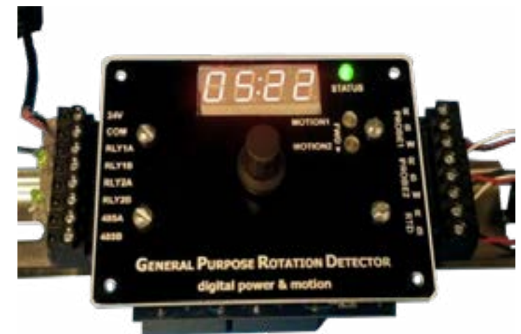
GPRD controller as installed on the electric panel.
