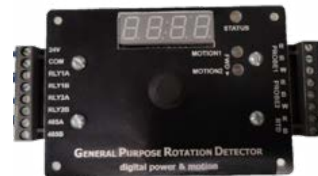
GPRD controller as installed on the electric panel.
