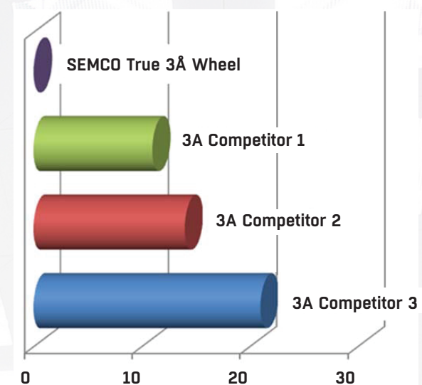
FIGURE 2. Measured Average Contaminant Carry-over Percentage 1 (%) of the True 3Å Wheel versus the competition.
